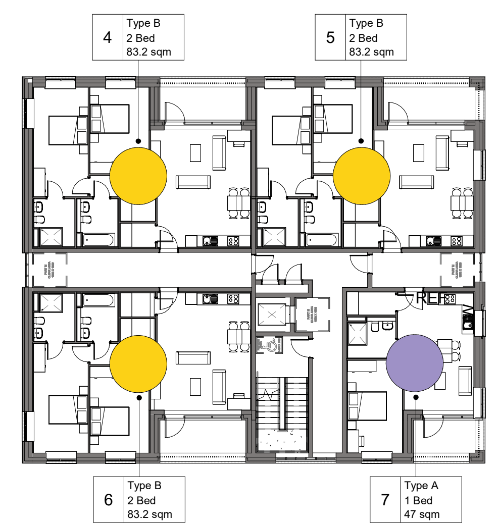
5 Apartment Block A First Floor - UD 1 : 200
