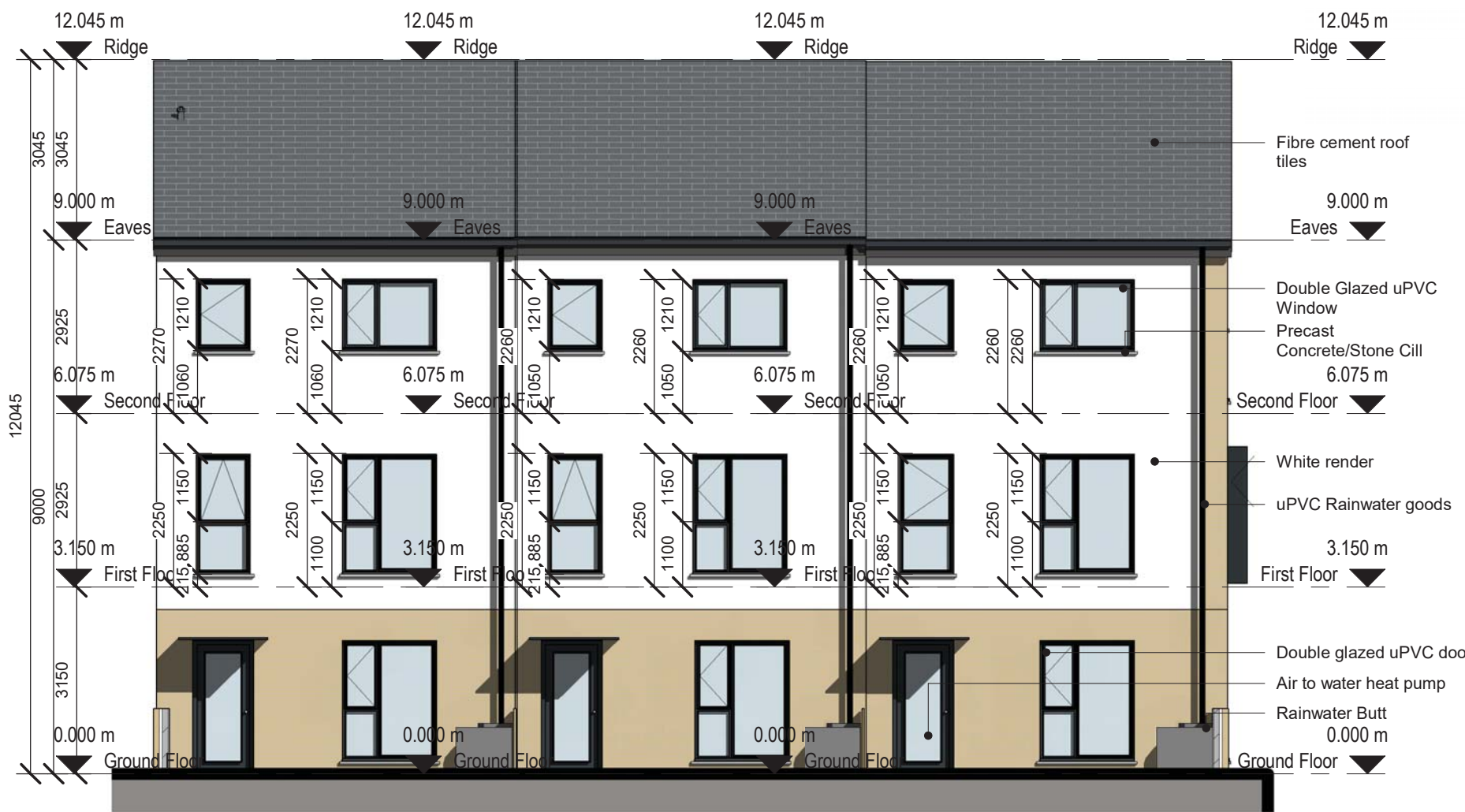
3 Duplex Rear Elevation - Types 1, 2 & 3 1 : 100
