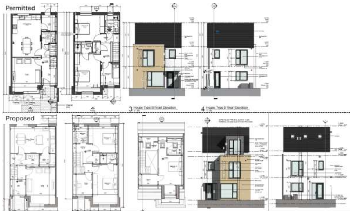
Figure 5. Previously Approved House Type B (top) and proposed House Type B (bottom)
