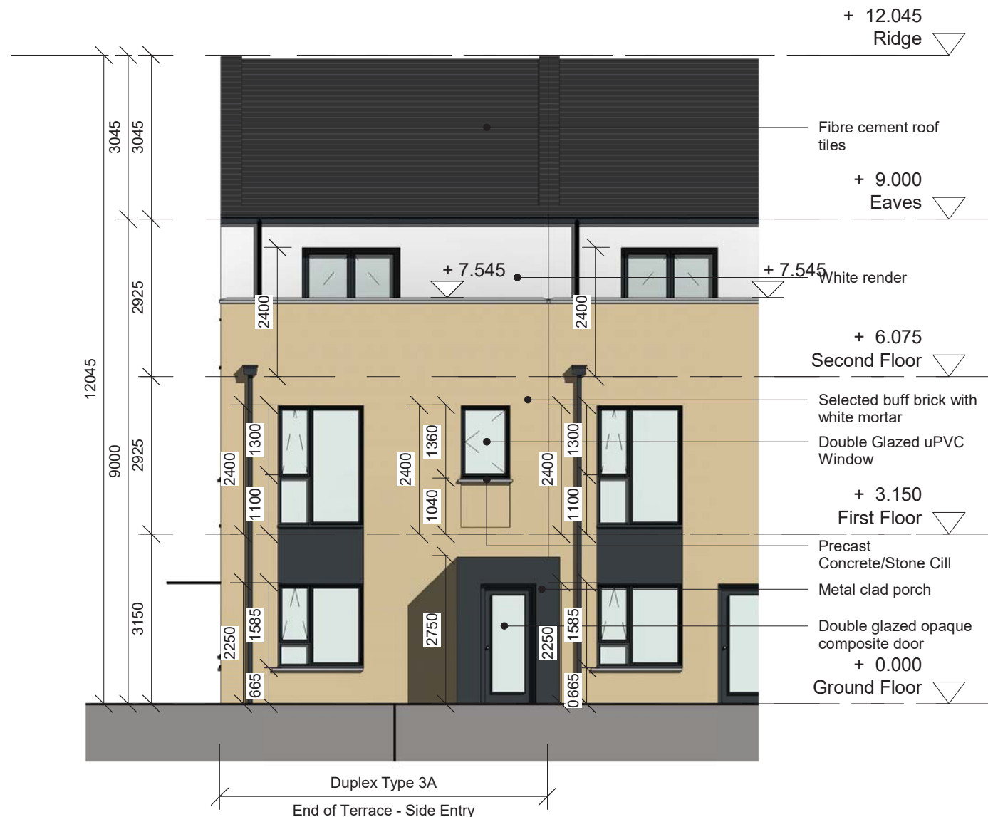
6 Duplex Front Elevation - Type 3A 1 : 100
