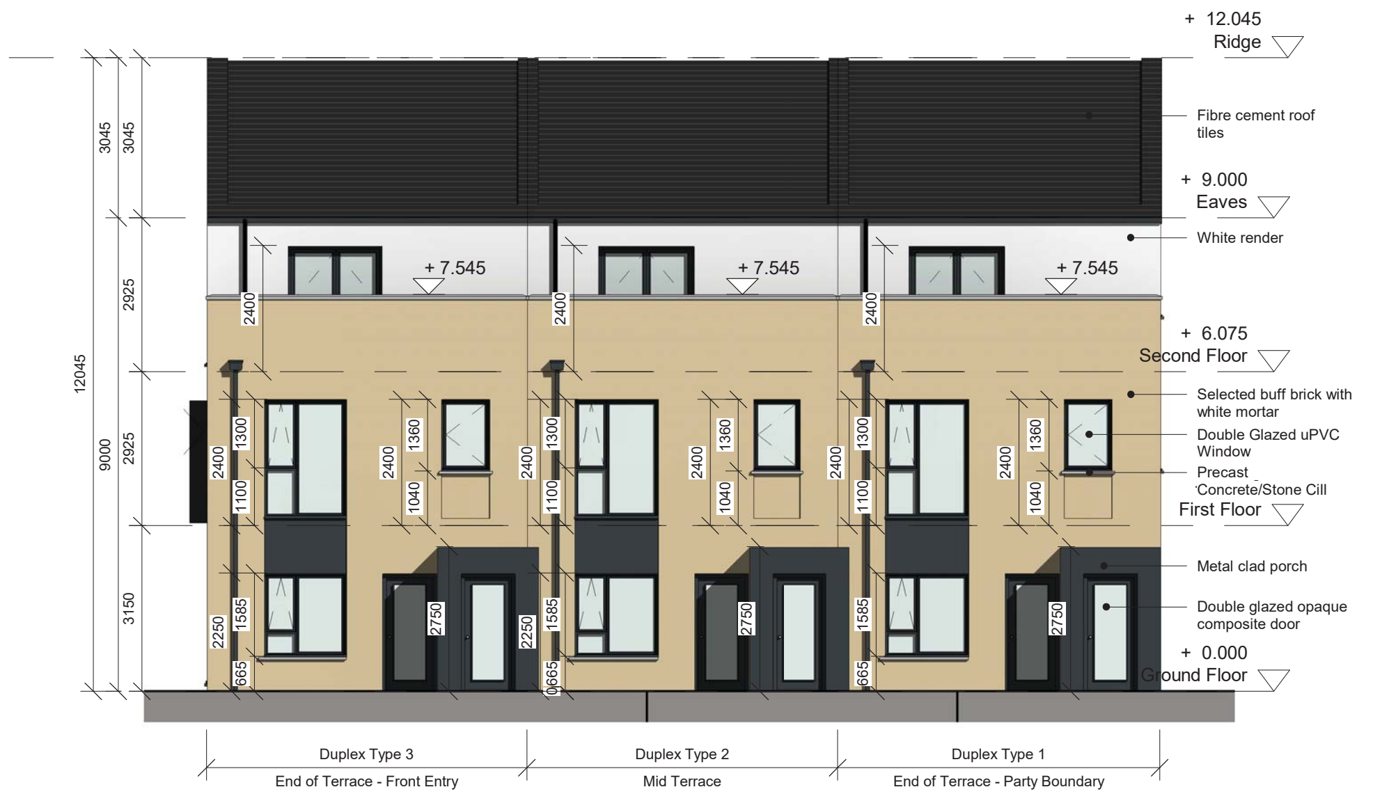
1 Duplex Front Elevation - Types 1, 2 & 3 1 : 100
