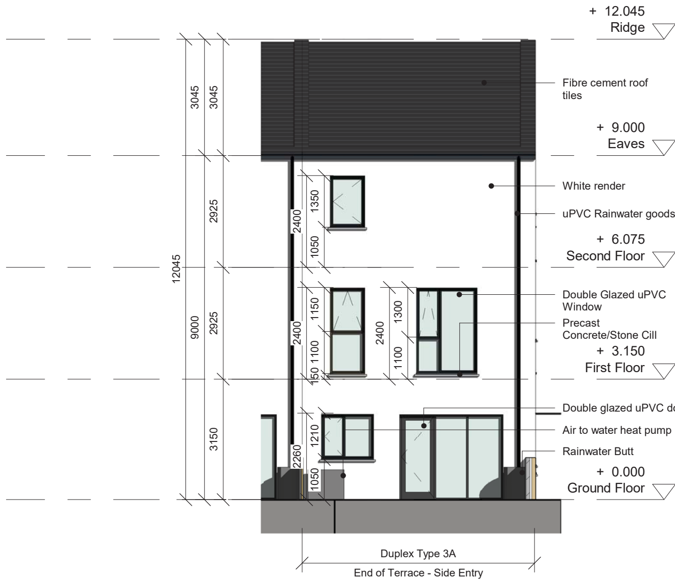
8 Duplex Rear Elevation - Type 3A 1 : 100
